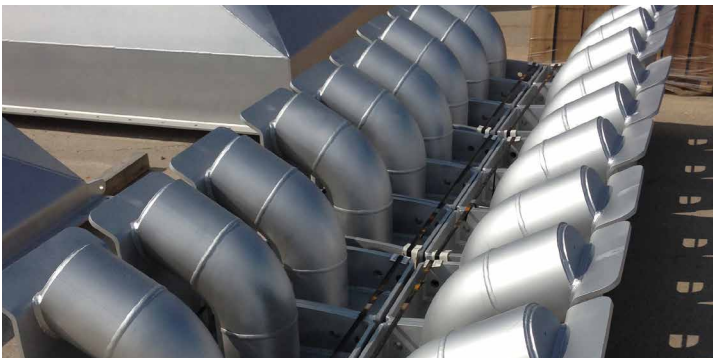
Ball and tube knockers ready for mounting
